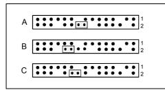
Pin pair A inserted = Skipping system and BIOS Setup password Pin pair B inserted = System BIOS recovery
